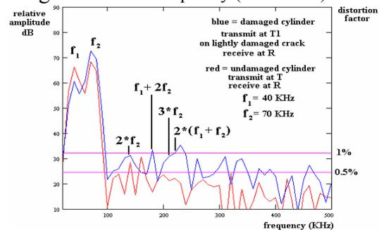
Figure 14 shows a spectral plot taken over the surface of a mildly damaged region of the concrete test cylinders, shown previously in Figure 4. This test was performed at the two frequencies 40 and 70 kHz. The two fundamental frequencies are not sufficiently separated to form clear spectral peaks, however the inter-modulation products and in particular the second multiple of  $f_1+f_2$  that is  $2*(f_1+f_2)$  shows a very clear peak above 1% distortion in the damaged region.
