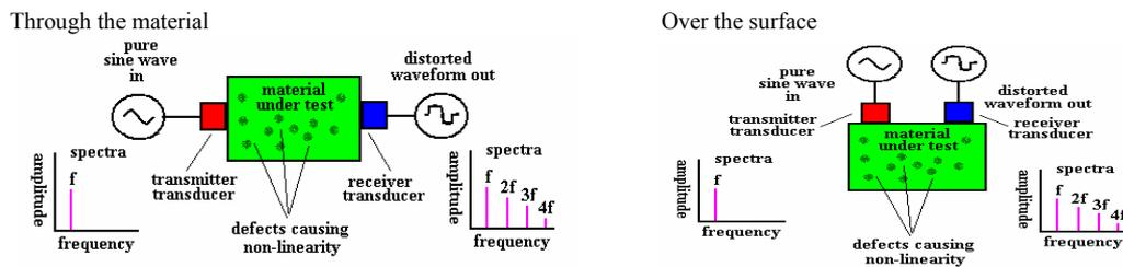
The harmonics are measured by examining the power spectra of the received signal. The transmitted frequencies (fundamental) amplitude is compared to that of the amplitudes of each of the harmonic frequencies. These harmonics are expressed in terms of decibels (dB) down from the fundamental, that is the number of decibels below the fundamentals amplitude. These values can be converted to a distortion factor that is expressed as a percentage.
