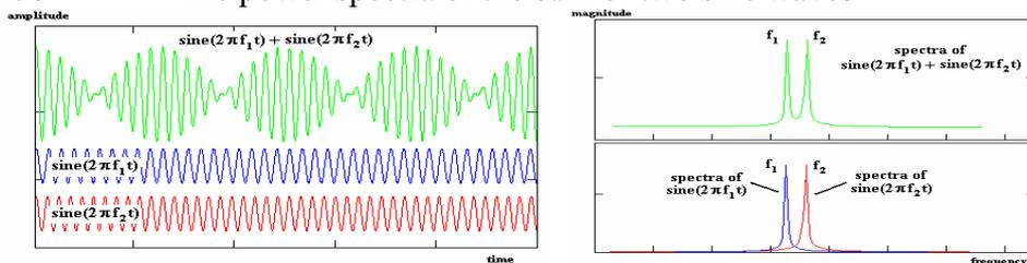
An ultrasonic wave composed of the sum of two sine waveforms of different frequencies,  $f_1$  and  $f_2$  with equal amplitude, can be represented by  $[\sin(a) + \sin(b)]$ , where  $a = 2\pi f_1 t$
