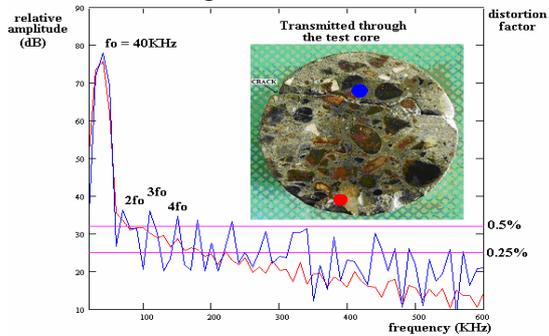
The photograph in Figure 7 shows a micro-damaged drilled test core with an ultrasonic transmitter on the right and a receiver on the left. The blue trace of the spectral plot in Figure 8 shows that transmitting and receiving in a line through the concrete close to the crack produces relatively high levels of 2<sup>nd</sup>, 3<sup>rd</sup> and 4<sup>th</sup>, harmonics above 0.5%. Transmitting and receiving in a line away from the crack (shown in red) produces little harmonic content.
