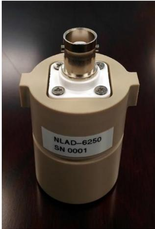
NLAD design of the narrowband transducer assembly consists of a piezoelectric epoxy composite material to a glass ceramic front face which is placed in contact with the concrete structure using a dry contact pad. These transducers can be used to both transmit and receive.
